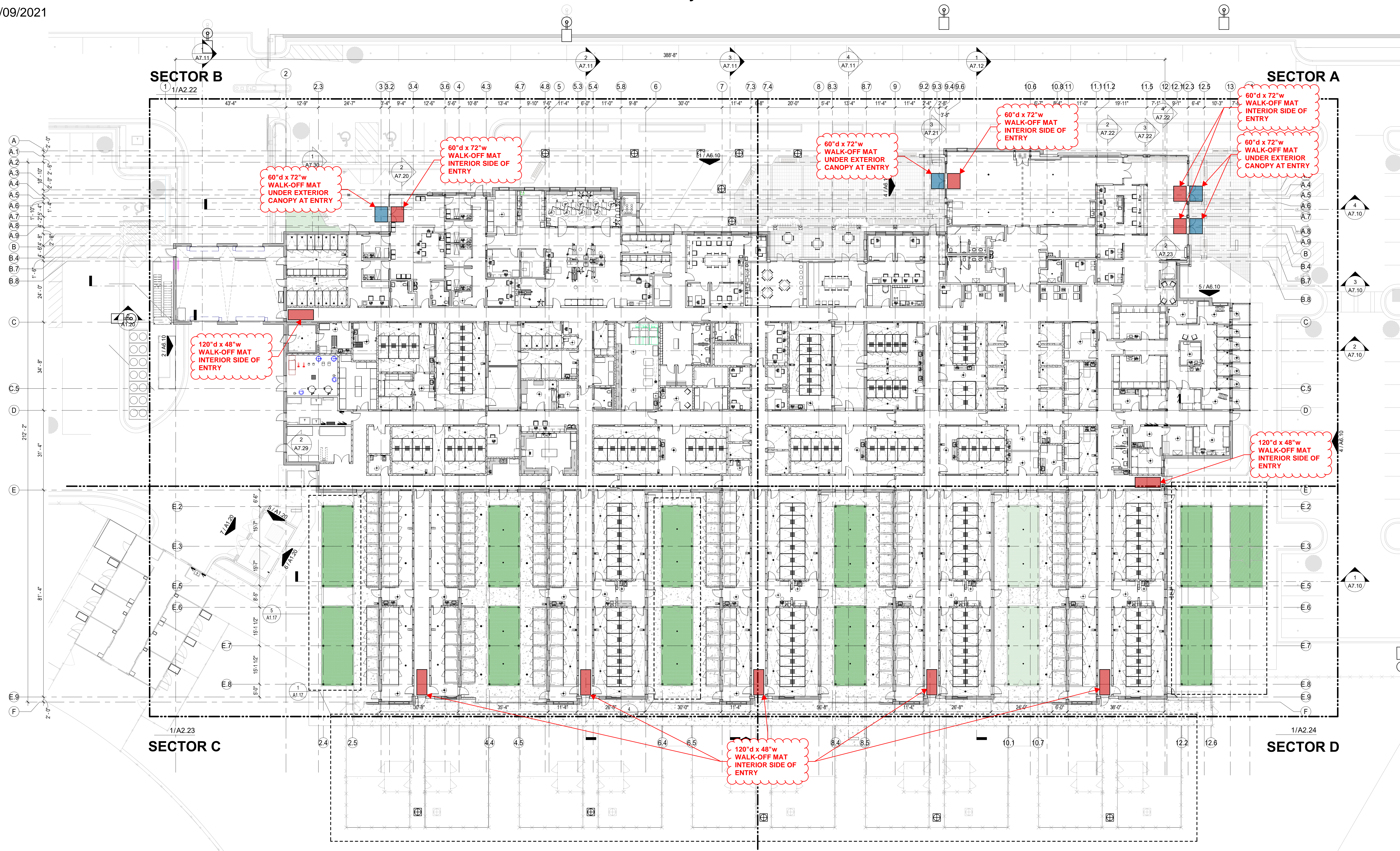
IEQc1 WALK-OFF MAT PLACEMENT DIAGRAM
